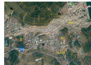
“Orthophotomap” compiling main items from Digital Japan Basic Map (map information) in ortho-image
